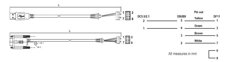
RS232 device needs external 5V power supply. This can be achieved either with an external power supply or via pin 9 of DSUB9 connector. The USB device is powered via USB connector.
